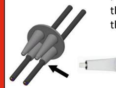
Pull cables through (use the lubricant)
