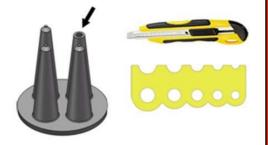
Cut endcap at ½ diameter of the cables – use cutting template
