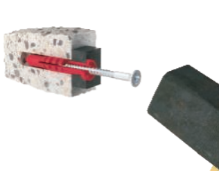
Hammer in concrete
